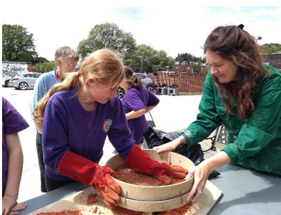
Sifting the special sand into the mould to create the pewter cast
